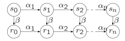
**C2** (Invisibility)  $ample(s) \neq enabled(s) \Rightarrow ample(s) \subseteq invisible(s)$ If s is not explored completely all transitions from ample(s) are invisible.
